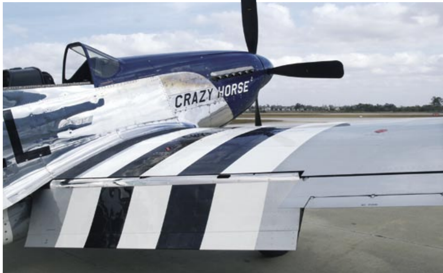
ABOVE The hydraulically actuated flaps are huge. (ALL KEY - DUNCAN CUBITT UNLESS STATED)
