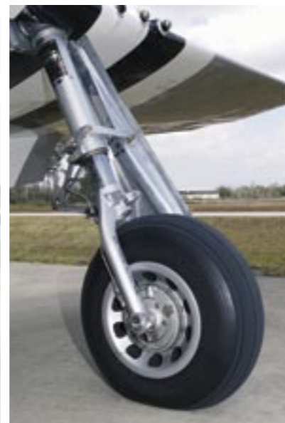
FAR LEFT As the mainwheels retract inwards, the undercarriage track is relatively wide.
