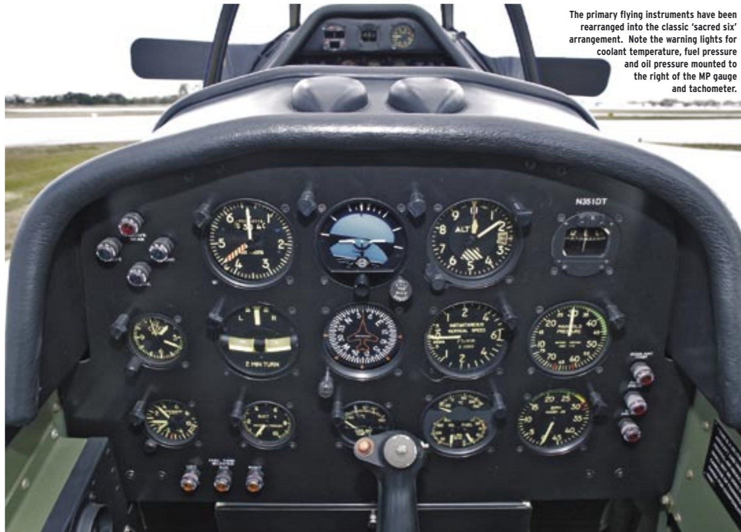
BELOW LEFT At first glance the front cockpit looks a bit cluttered, but closer inspection shows it to be very well-designed, with the various systems and sub-systems all laid out logically.
