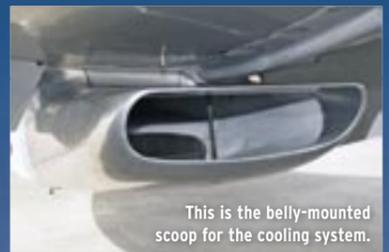
This is the belly-mounted scoop for the cooling system.
