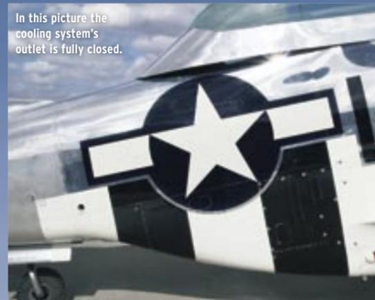
In this picture the cooling system's outlet is fully closed.
