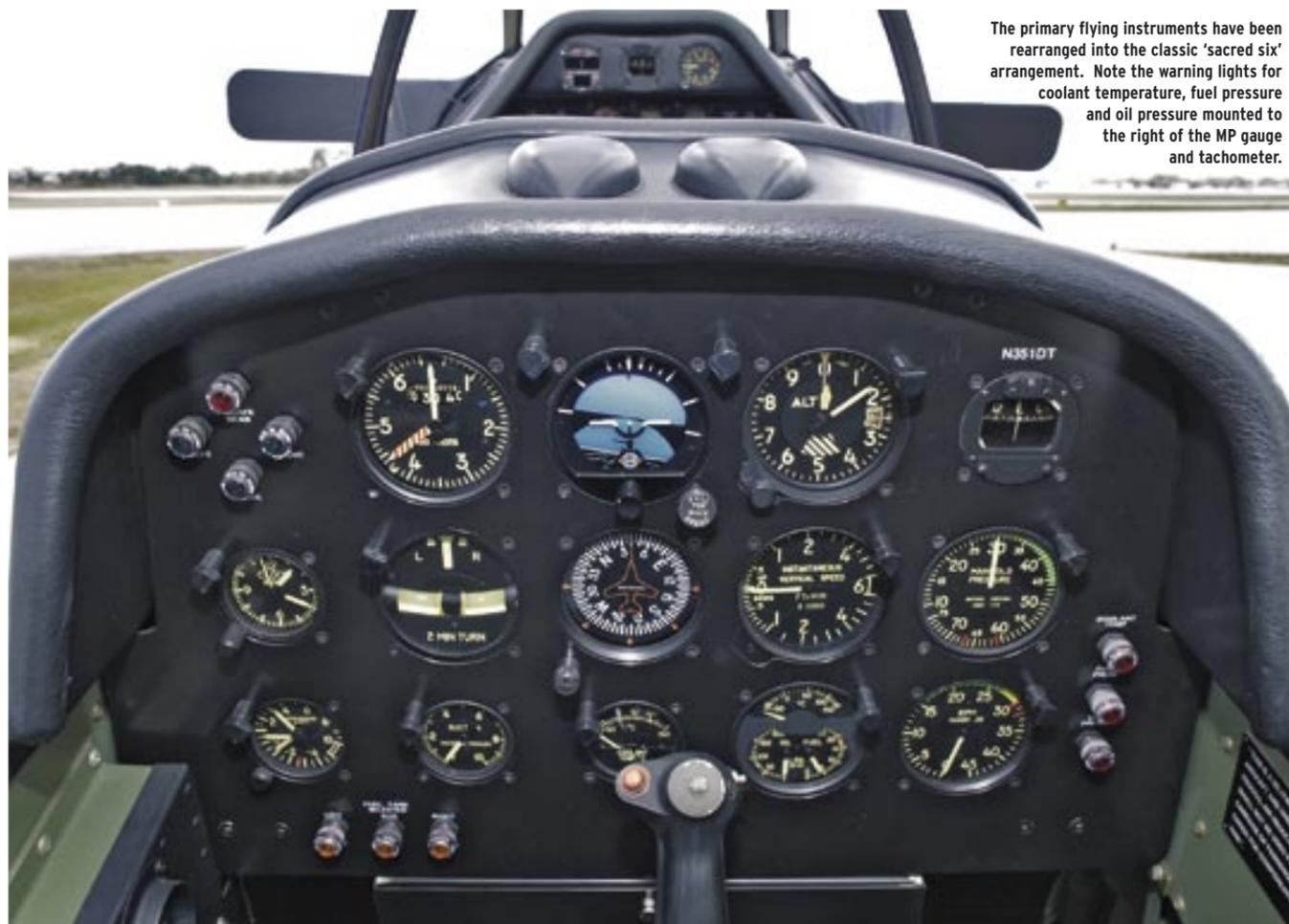
The primary flying instruments have been rearranged into the classic 'sacred six' arrangement. Note the warning lights for coolant temperature, fuel pressure and oil pressure mounted to the right of the MP gauge and tachometer.
