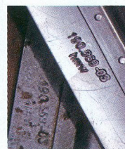
ABOVE An original inspection-hatch cover with part number stamping in the background, with an exact duplicate of the original part, including the stamping, in the foreground.
